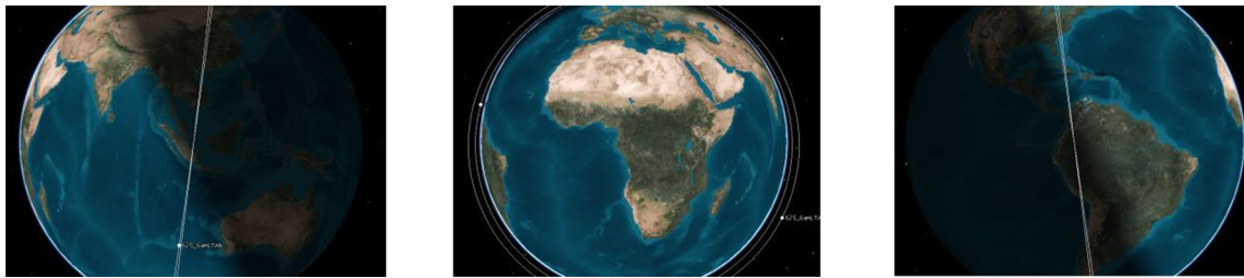
Fig. 7 Orbital plane (400 and 600 km altitude) for a dusk/dawn orbit at winter solstice (left and center) and summer solstice
