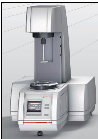
Figure 25: Picture of a MCR 302 rotational rheometer from Anton Paar used for this study [37, 70].
