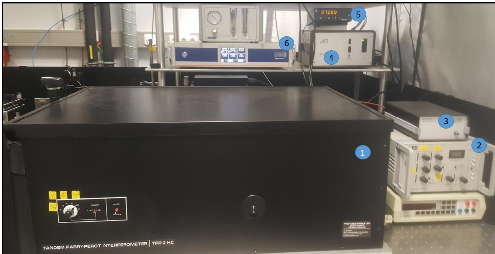
Figure 1: Picture of the tandem Fabry-Perot spectrometer (1) with corresponding electronics. (2) Control unit of the spectrometer, (3) Energy supply of the photon-counter, (4) control unit of the isolation stage, (5) mirror separation distance control unit and (6) the temperature controller for additional temperature measurements.
