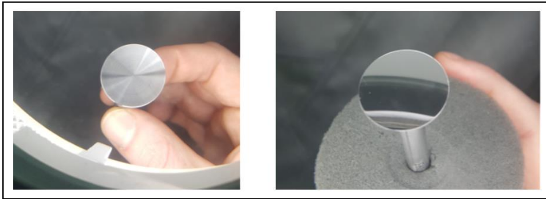
Figure 99: Picture of PP25 geometries, left a common plate-plate geometry where the rings of manufacturing are still visible; right, the polished PP25 geometry used in further experiments.
