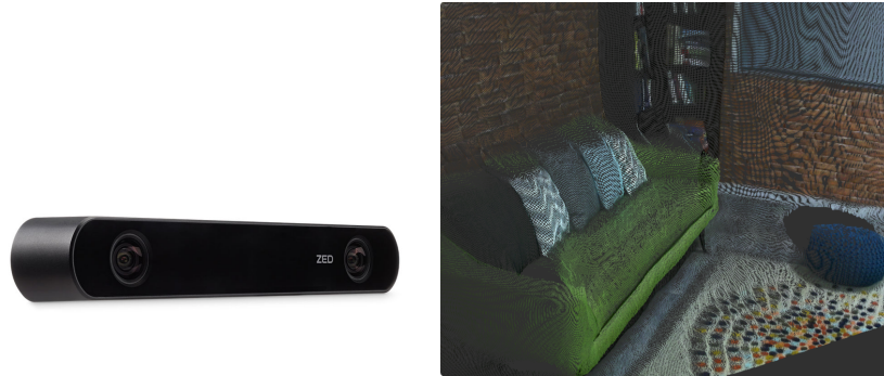
Figure 1.1: Zed stereo camera and generated pointcloud.
