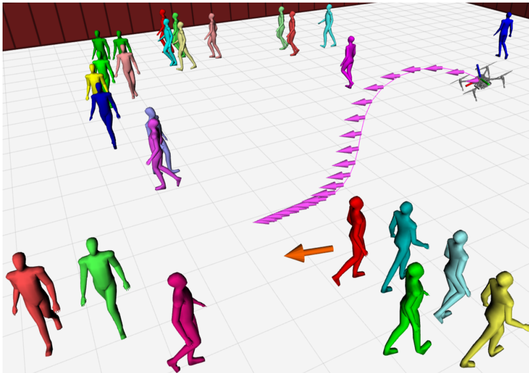
Figure 6.6: Crowd collision avoidance simulation with 30 pedestrians. The orange arrow represents the moving reference position. The robot pose and predicted trajectory are indicated by the frame and the purple arrows respectively.
