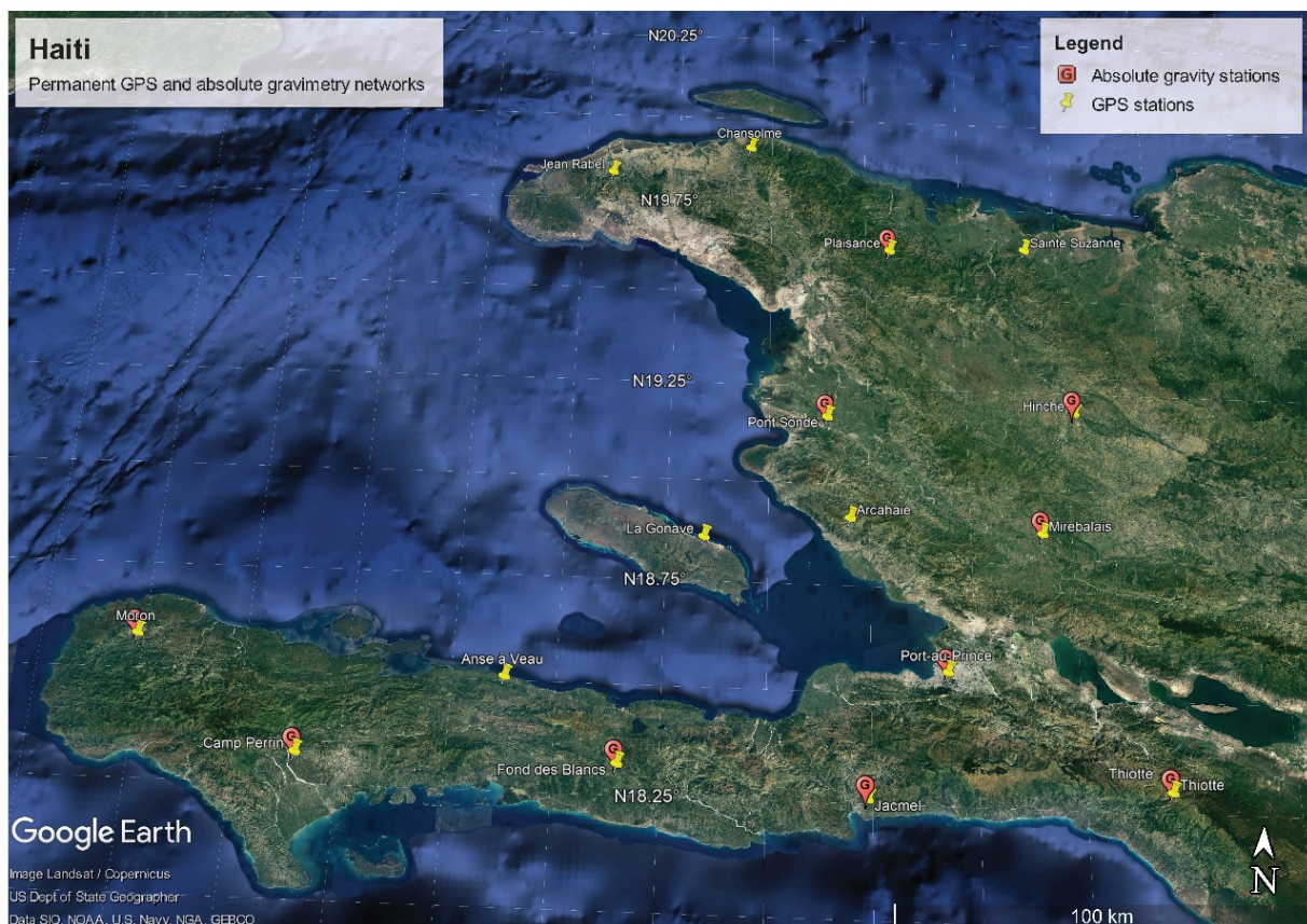
Figure 1. Locations of the 16 permanent GPS stations (yellow) of the CNIGS and of the 10 established absolute gravity stations (red).
