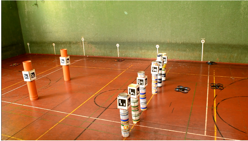
Fig. 1 Experimental flight of a basic instance of the framework “CVG Quadrotor Swarm”. This basic instance is characterized by swarm behavior, using 5 AR Drones. The row of columns represents a virtual wall with a single 1.5 m opening in the middle. In order to simplify the localization problems the columns are marked using ArUco visual markers [5]. In this flight the mission of the swarm is to cross from one side to the other, while each swarm agent also has to avoid collision with the columns and the other drones. This test was designed to showcase the capabilities of this basic instance of the framework.
