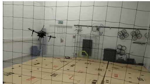
Fig. 8: Our aerial robot flying autonomously inside our flight arena during an experimental validation test. A video with several real flight experiments can be visualized in: https://youtu.be/peR2cTX02Ww .
