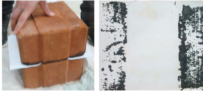
Figure 10. Identification of the actual contact area using a carbon footprint paper [49]
