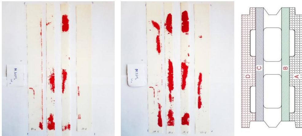
Figure 98. Actual contact area in the bed-joints of the DSM prims with raw block units, at 5% and 15% of F_{u, \text{Block}}
