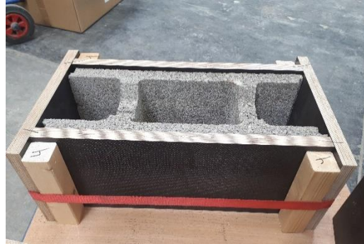
Figure 44. Sample of the wood formwork used to apply the contact layers [122]
