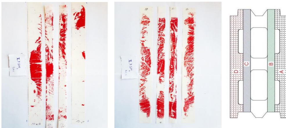
Figure 99. Actual contact area in the bed-joints of the DSM prims with improved block units, at 5% and 15% of F_{u, \text{Block}}
