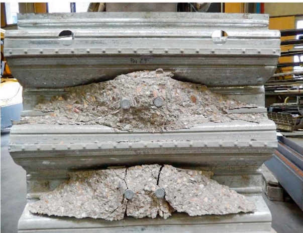
Fig. 2. Concrete cones observed in the push-out specimen after demounting.
