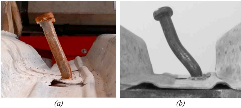
Fig. 3. Plastic deformation of the stud with (a) one and (b) two plastic hinges.
