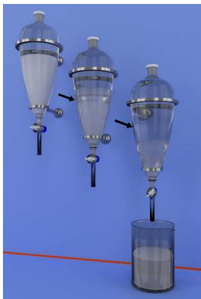
Figure 4.6: Schematic illustration of the separation of the LC fraction from the isotropic phase using a separatory funnel. A CNC suspension is filled into a separatory funnel (first funnel). A sharp boundary between phases is clearly visible after two weeks (second funnel). Finally, the stopcock is opened and most of the LC phase is drained out, closing the valve before reaching the interface with the isotropic layer (third funnel).
