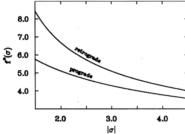
Fig. 2. Viscous drag factor  $f^e(\sigma)$  plotted as a function of  $|\sigma|$ .  $\sigma$  is positive for the retrograde equatorial mode, negative for the prograde equatorial mode. The asymmetry of the drag factor provides a natural redundancy check on the viscosity recovered from the two equatorial translational modes of the inner core.
