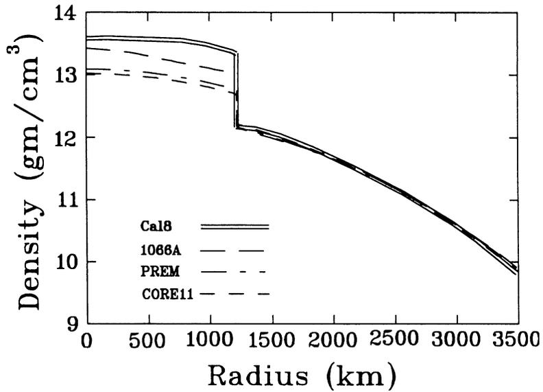
Fig. 4. Density profiles in the inner and outer cores for Earth models Cal8, 1066A, PREM and Core11. They show little difference in the outer core but range over about 4.4% in inner core density.
