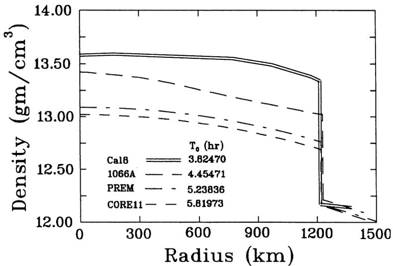
Fig. 5. Detailed density profiles in the inner core for Earth models Cal8, 1066A, PREM and Core11. The  $0.6 \text{ gm} \cdot \text{cm}^{-3}$  density range causes nearly a 2 h difference in the unsplit period  $T_0$ .
