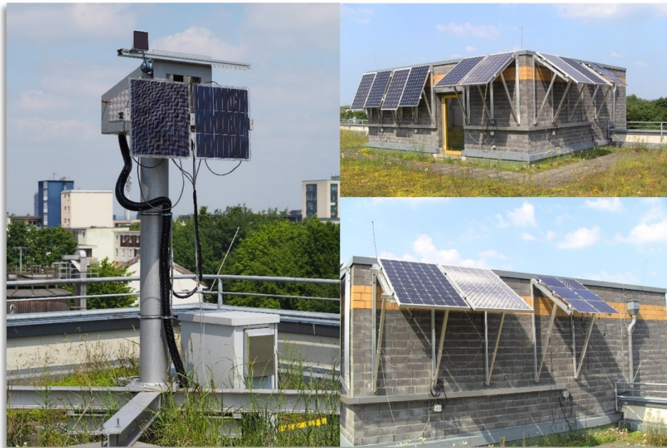
Fig. 2.6: Left: Solar tracking system at the Cologne University of Applied Sciences. Right: Outdoor measuring station for the continuous determination of the module performance. The module tilt angle can be varied. The door is oriented to the east.
