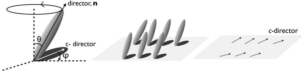
Figure 2.2 c -director in SmC phase. (a) Determination of the c -director as a unit vector by projecting the director \mathbf{n} onto the smectic layer plane. (b-c) The c -director field in a single layer of SmC.
