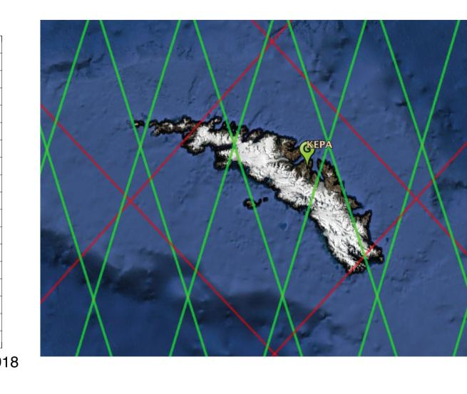
Figure 7: KEP tide gauge and satellite altimetry mission ground tracks for TOPEX/POSEIDON/-JASON (red lines) and Sentinel-3 (green lines for future reference).
