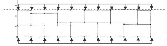
**Figure 4: Randomly chosen blocks with different heights and dry-stacked with stretcher bond.**
