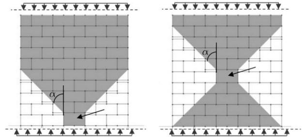
**Figure 5: Visualisation of load-transmission in a dry-stacked wall structure using the above mentioned algorithm.**
