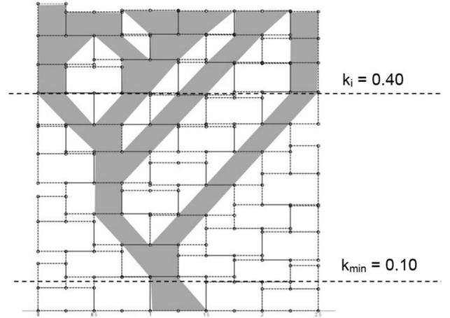
**Figure 12: Example of effective area calculation for the determination of the stress state in the dry-stacked masonry.**
