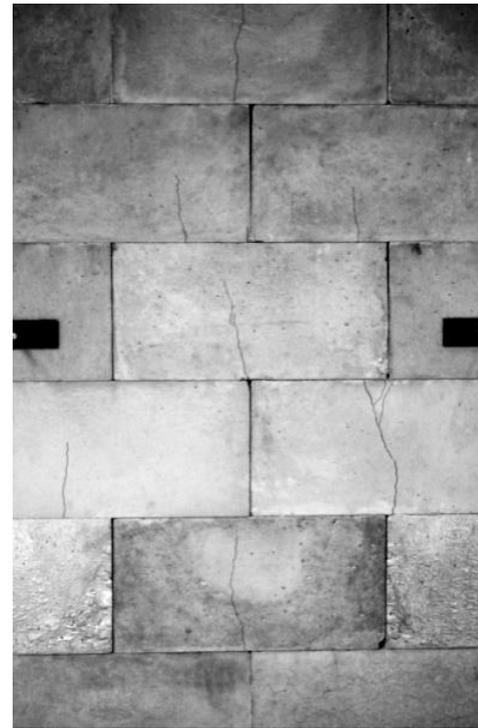
**Figure 18: Characteristic crack patterns observed during experimental investigations involving vertical loadings and bending moments on stretcher-bonded and dry-stacked masonry structures.**
