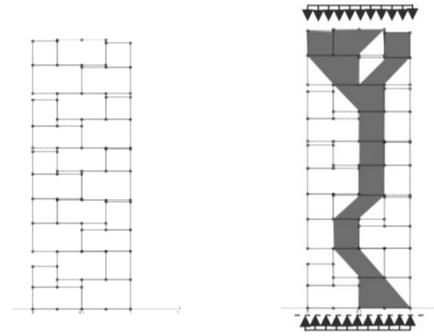
**Figure14: Numerical modelling of a 1.0 x 2.5 m dry-stacked wall (height differences between adjacent elements exaggerated for visualisation purposes).**
