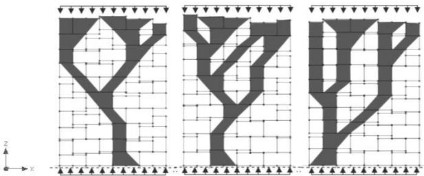
Figure 8: Load percolation in wall structures of 2.50 m height and  $L = 2.00$  m length.
