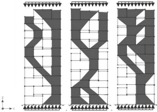
Figure 7: Load percolation in wall structures of 2.50 m height and  $L = 1.00$  m length.
