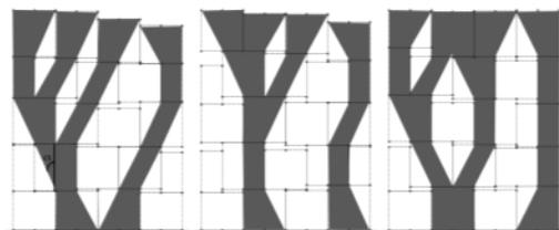
**Figure 19: Load distribution in 2.00 m long and 2.50 m height structures.**
