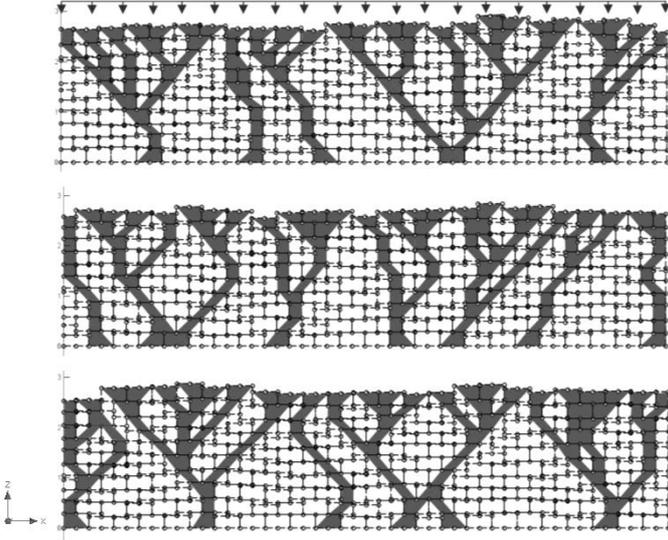
**Figure 11: Vertical load transfer and distribution in a wall structure of ~2.50 m height and L = 12.00 m length, with amplified standard deviation of 0.02 m in height of randomly selected blocs (Agaajani et al., 2015).**
