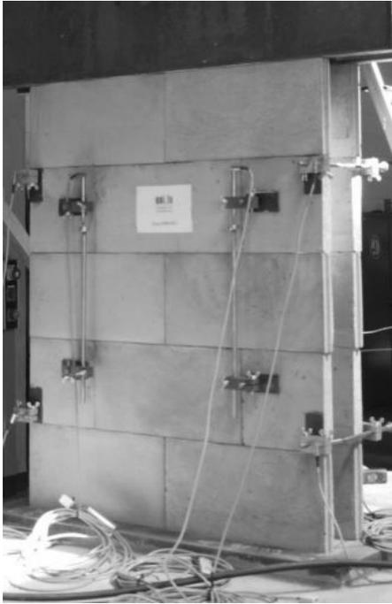
Figure 1: Dry-stacked masonry (Agaajani et al., 2015).
