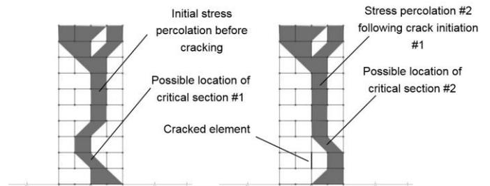
**Figure 15: Comparison between initial stress distribution (left) and new stress distribution after cracking of the critical section #1 (right).**
