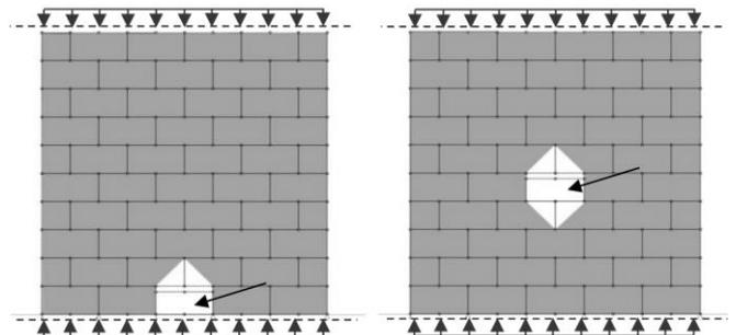
**Figure 6: Influence of reduced block height on load transmission in dry-stacked wall systems**
