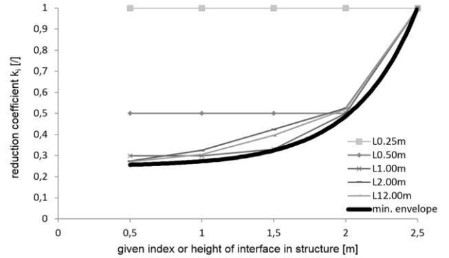
Figure 22: Reduction coefficient and minimum envelope of loaded area at a given index or height in dry-stacked structure of 2.50 m height and for different lengths (n=5).
