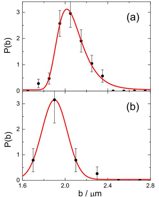
FIG. 3. Distributions of the minor axes lengths  $b$  of colloidal ellipsoids, as obtained by SEM for: (a)  $\lambda_m = 1.4$ , (b)  $\lambda_m = 1.9$ , corresponding to Fig. 2(a) and Fig. 2(b), respectively. The distribution peaks at  $b = 2.02 \mu m$  for (a) and at  $b = 1.68 \mu m$  for (b), corresponding to  $t = 1.68 \pm 0.02$  and  $t = 2.02 \pm 0.02$ , respectively. The solid curves are fits by the Gumbel probability density function.
