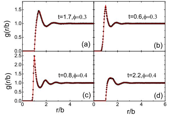
FIG. 8. The radial distribution functions of fluids of hard spheroids, obtained by Monte Carlo simulations (symbols) are perfectly matched by the PY-theoretical calculations (solid curves). The data are shown for different volume fractions  $\phi$  and aspect ratios  $t$  (see labels), both for the oblate and the prolate particles. The  $r$  values are normalized by the equatorial axis of the ellipsoids  $b$ .
