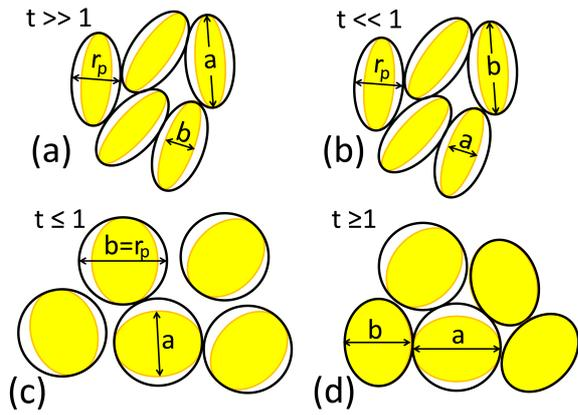
FIG. 9. Schematic representation of four different regimes of packing in fluids of spheroids: (a)  $t \gg 1$ ; (b)  $t \ll 1$ ; (c)  $t \leq 1$ ; (d)  $t \geq 1$ . Particle cross-sections are shown in yellow; the excluded volumes are depicted as black ellipses and circles.  $r_p$  is the position of the principal peak of the  $g(r)$ ;  $a$  is the symmetry axis.
