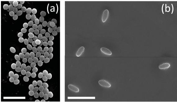
FIG. 2. SEM images of prolate colloidal ellipsoids, for the PDMS matrix stretched to an extension ratio of (a)  $\lambda_m = 1.4$ , (b)  $\lambda_m = 1.9$ . Note, the particles in panel (a) are oriented at different angles to the substrate, so that the apparent aspect ratios are smaller than the actual ones. Panel (b) was obtained by stitching of two separate SEM images, as marked by the horizontal black line.
