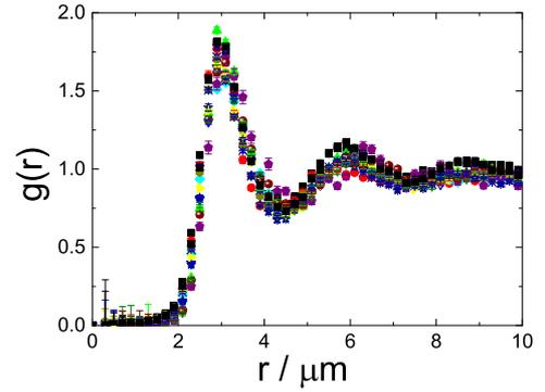
FIG. 6. The radial distribution functions (RDF) obtained from 2D slices, at different positions within the sample (different symbols), perfectly overlap. Here the aspect ratio and the volume fraction of the particles are  $t = 1.68$  and  $\phi = 0.21$ , respectively.
