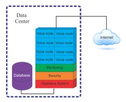
Fig. 2. Single cloud VoiP architecture.
