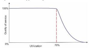
Fig. 5. Voice quality versus processor load (utilization).
