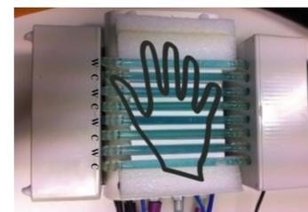
Figure 3: Custom-built thermal grill device. (W: warm tubes; C: cold tubes)
