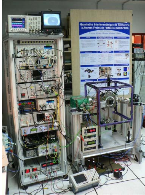
Figure 1.11: Atom gravimeter from ONERA. Although the set-up is compact, the electronics is bulky.
