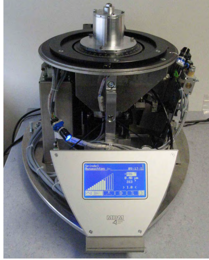
Figure 4.16: Balancing machine BMT 200 S (modified) with the mounting jig for balancing around X - and Y -axis mounted.
