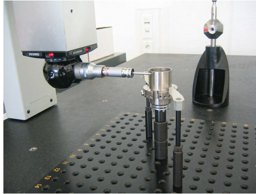
Figure 4.4: The position of the OC is measured with a coordinate measuring machine.
