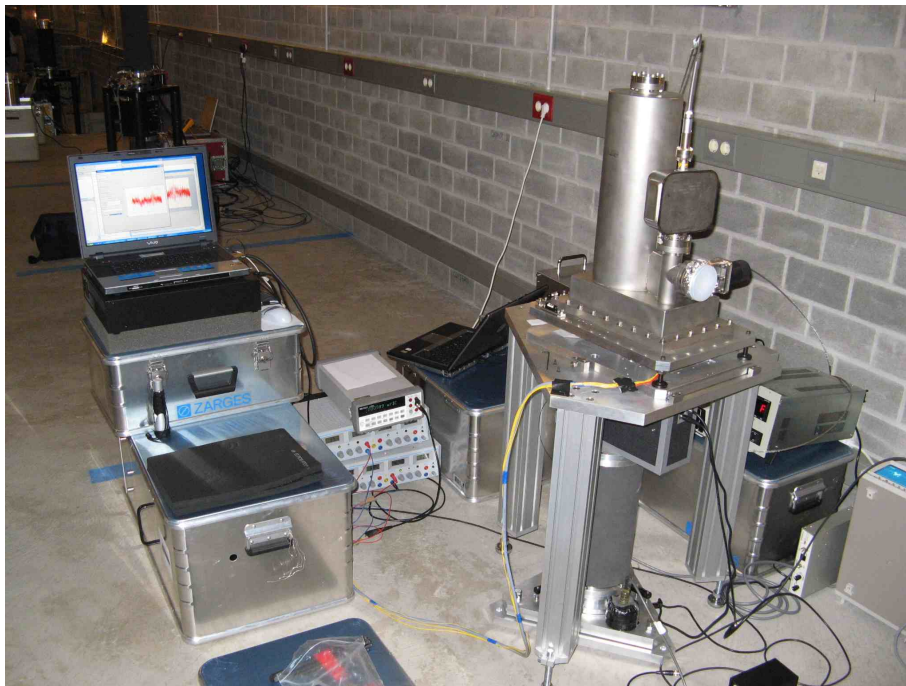
Figure 3.1: The setup of the portable free fall gravimeter MPG-2 at a measurement point in the mine in Walferdange/ Luxembourg in November 2007. (The position of the ion pump is different in the new setup - see discussion in Subsection 3.3.1).
