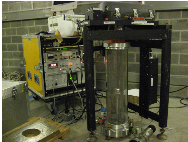
Figure 1.10: The picture shows the rise and fall gravimeter IMGC#2 of the Institute of Metrology G. Colonnetti, Italy, at the international comparison of absolute gravimeters in Walferdange, Luxembourg, November 2007.
