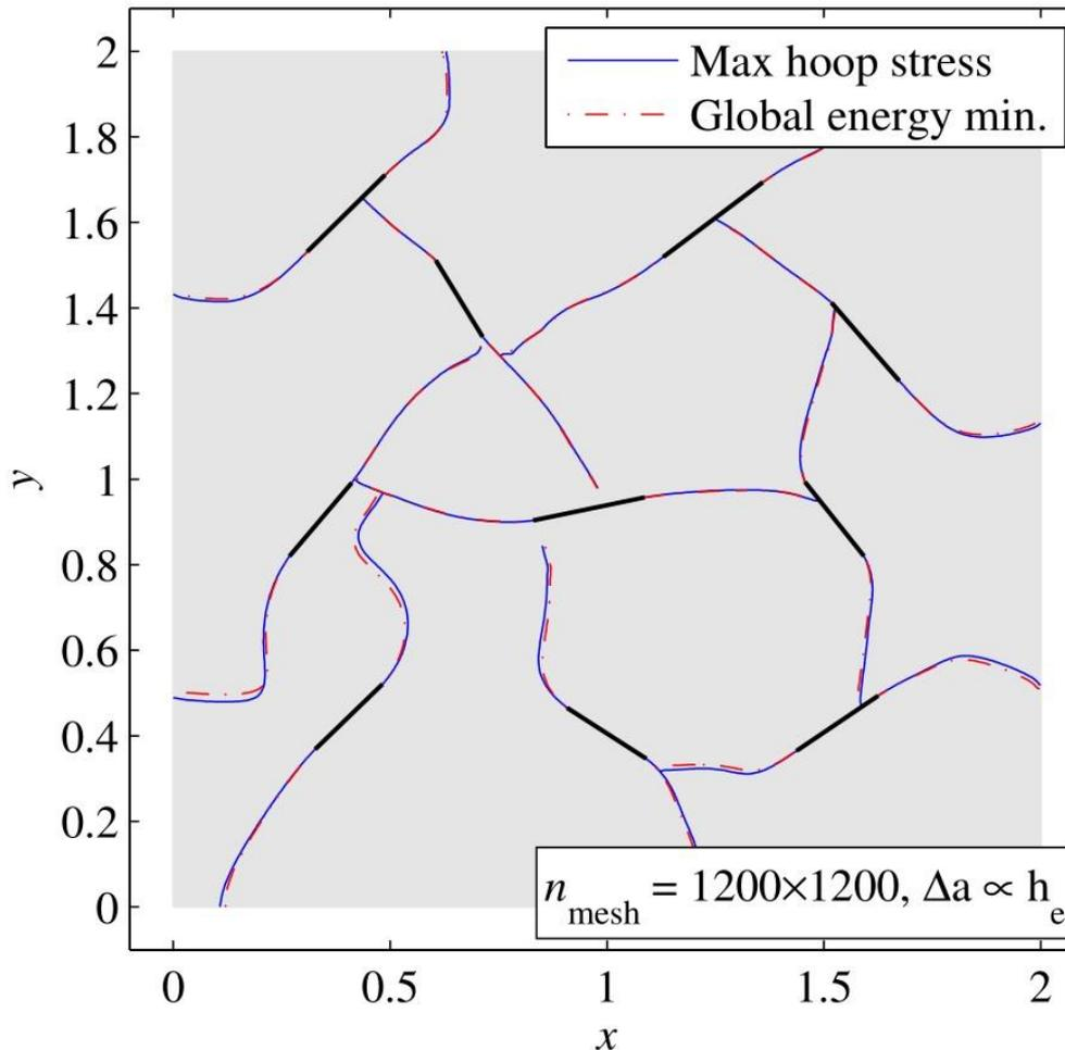
**Convergence to same fracture path by hoop–stress and energy–min. criteria**
