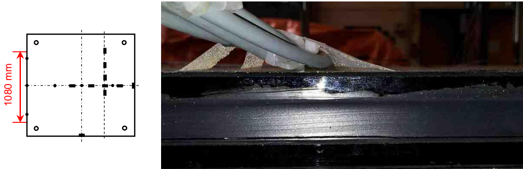
Figure 9.48 Location and rupture of the silicone sealant close to the inner glass pane
