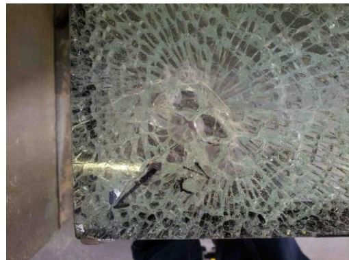
Figure 9.52 Failure of the connection
