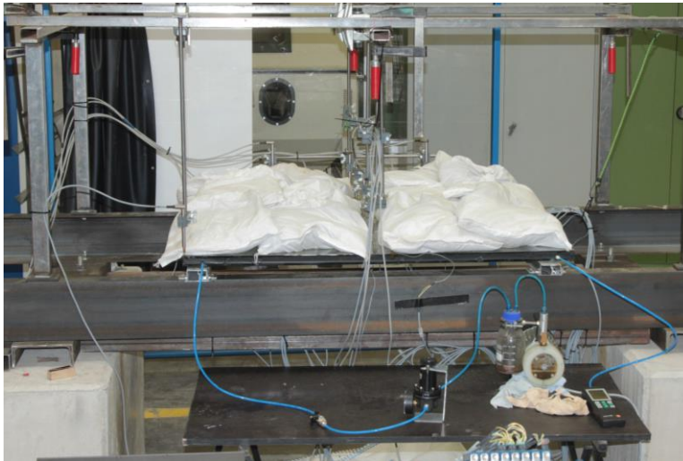
Figure 9.45 Gap in the centre of the IGU for the installation of the displacement sensors along path 0
