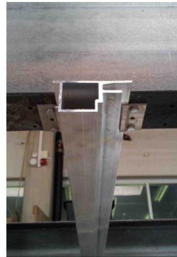
Figure 9.5 Connection of the aluminium bars to the U-profiles
