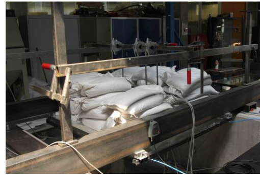
Figure 9.9 Sandbags on inner glass pane (Configuration 2)
