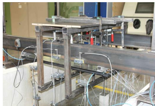
Figure 9.11 Steel frame with wooden plate for the loading of the outer pane
