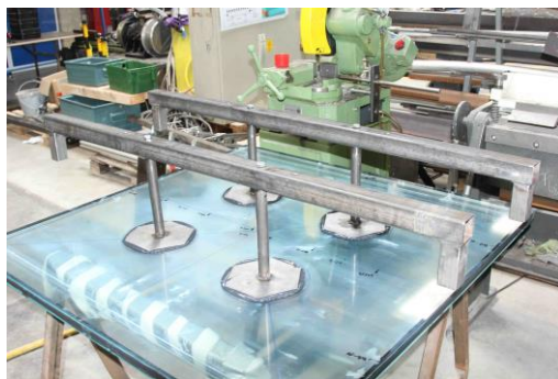
Figure 9.10 Connection of the steel frame to the outer pane
