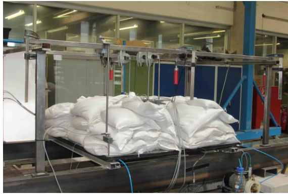
Figure 9.21 The wind pressure load applied with sandbags
