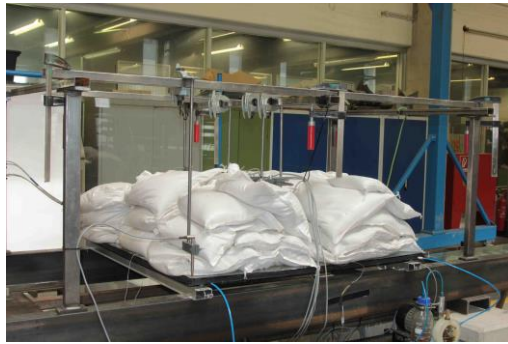
Figure 9.8 Sandbags on outer glass pane (Configuration 1)
