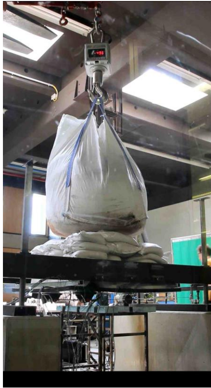
Figure 9.56 Application of failure load
