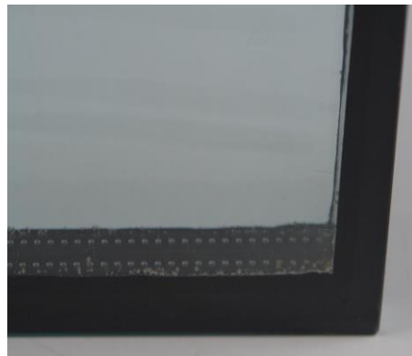
Figure 2.23 Corner of an insulation glass unit
