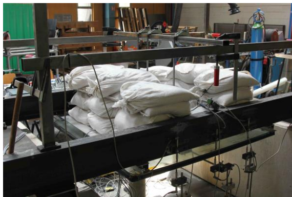
Figure 9.23 Sandbags on the inner pane
