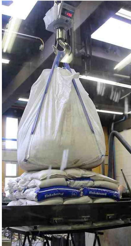
Figure 9.51 Failure load applied with sandbags
