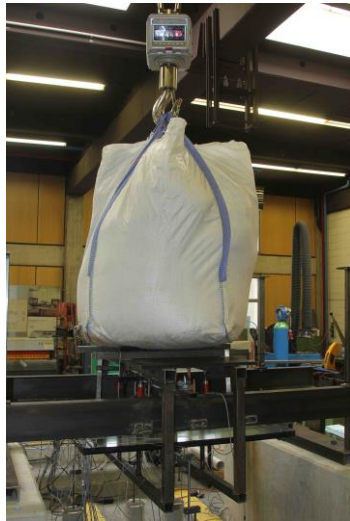
Figure 9.25 Loading of the outer glass pane with a sandbag
