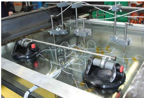
Figure 9.15 Assembling for the application of the self-weight
