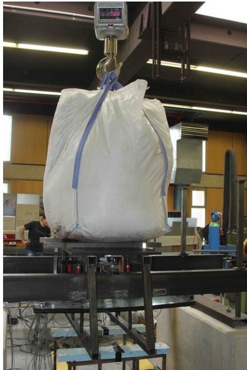
Figure 9.60 Application of wind suction load
