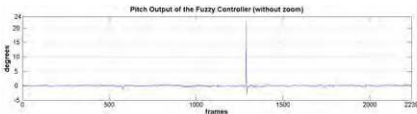
Fig. 26. Response of the Fuzzy control for the Pitch axis of the visual platform tracking a dynamic object (a van).
