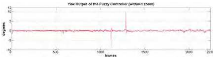
Fig. 25. Response of the Fuzzy control for the Yaw axis of the visual platform tracking a dynamic object (a van).
