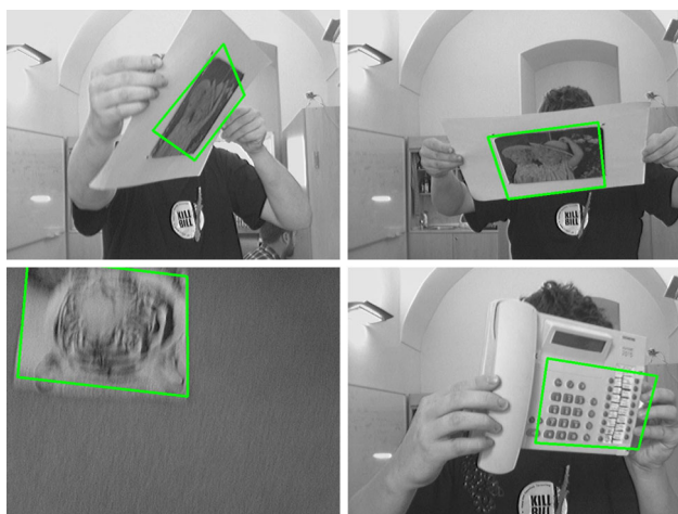
Fig. 19 Loss-of-locks of the HMPMR-ICIA. The first row shows the results of the MOUSEPAD sequence; and the second and third rows show the results of the TOWEL and the PHONE sequences, respectively
