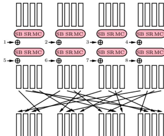
Running two instances of AESQ in parallel yields highest throughput on Haswell processors.
