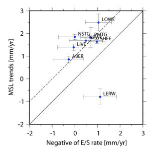
Figure 1: MSL trends for eight tide gauges compared with the negative of the emergence/submergence (E/S) rates based on CGPS and AG.
