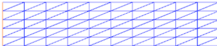
Figure 2: Mesh of the beam
