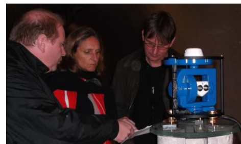
Figure 3: ZAMG scientists with Eng. Bracke, making a point during the installation of AUTODIF. Note the blue housing protecting the instrument from dust and humidity.
