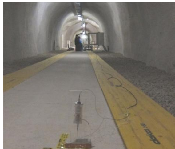
Figure 2: CDSM measures the Earth's magnetic field at the geomagnetic Conrad Observatory.
