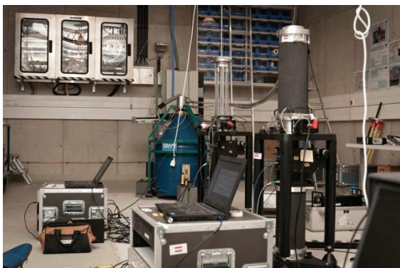
Figure 1: Absolute gravimeters side-by-side with the superconducting gravimeter at the Conrad Observatory (FG5-242 from Austria, FG5X-216 from Luxembourg with the glass tube and SG GWR C025).
