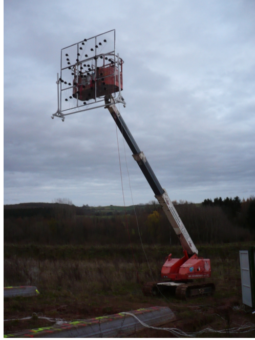
Figure 3.2.: Beamforming grid fixed to a cherry picker
