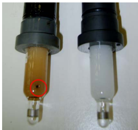
Fig. G.1 ORP electrodes – after 3 months in biogas reactor and a new one before use; red marked the critical diaphragm opening – a place of microbial growth
