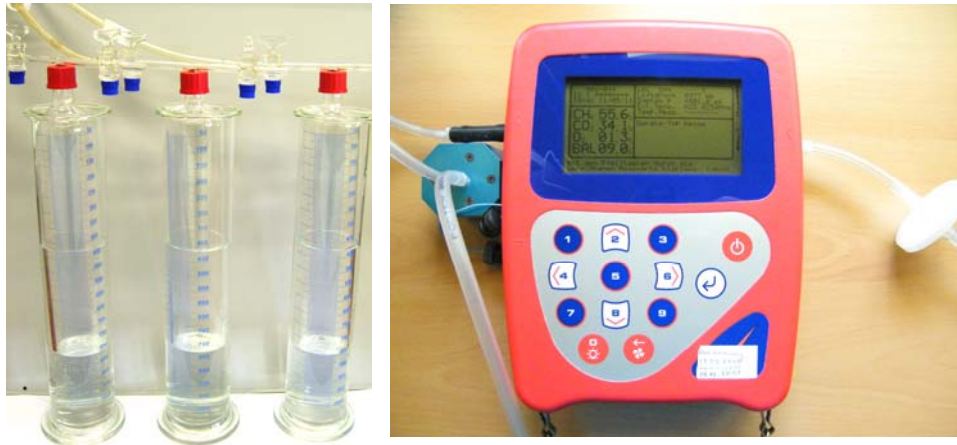
Fig. 3.7 The gas meters (left) and the biogas monitor (right) used in the studies
