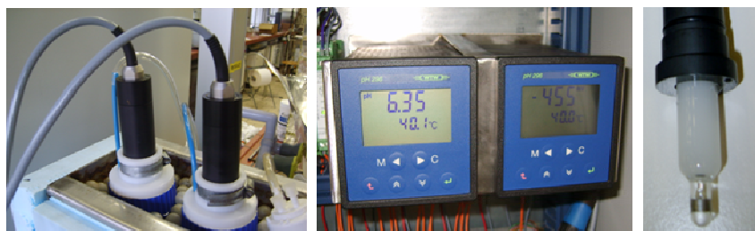
Fig. 3.6 ORP and pH on–line system applied in the test: the electrode adapters in the fermenters (left), the monitoring displays (central), an ORP electrode (right).
