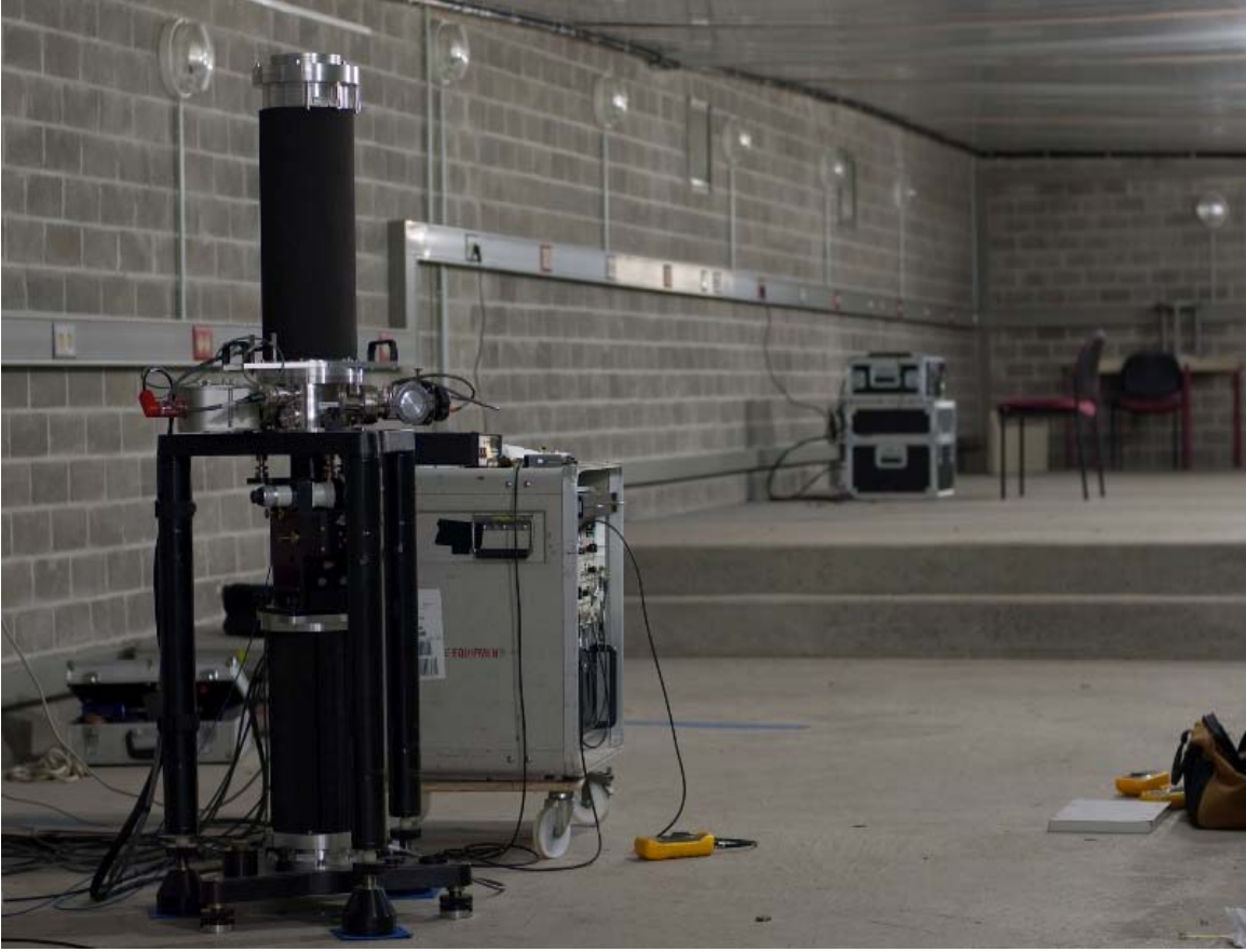
Fig. 3.17: The free-fall absolute gravimeter FG5 located in the WULG at a few meters distant from the OSGCT40. The absolute gravity measurements provided by the FG5 have been used to assess the drift of the superconducting relative gravimeter.
