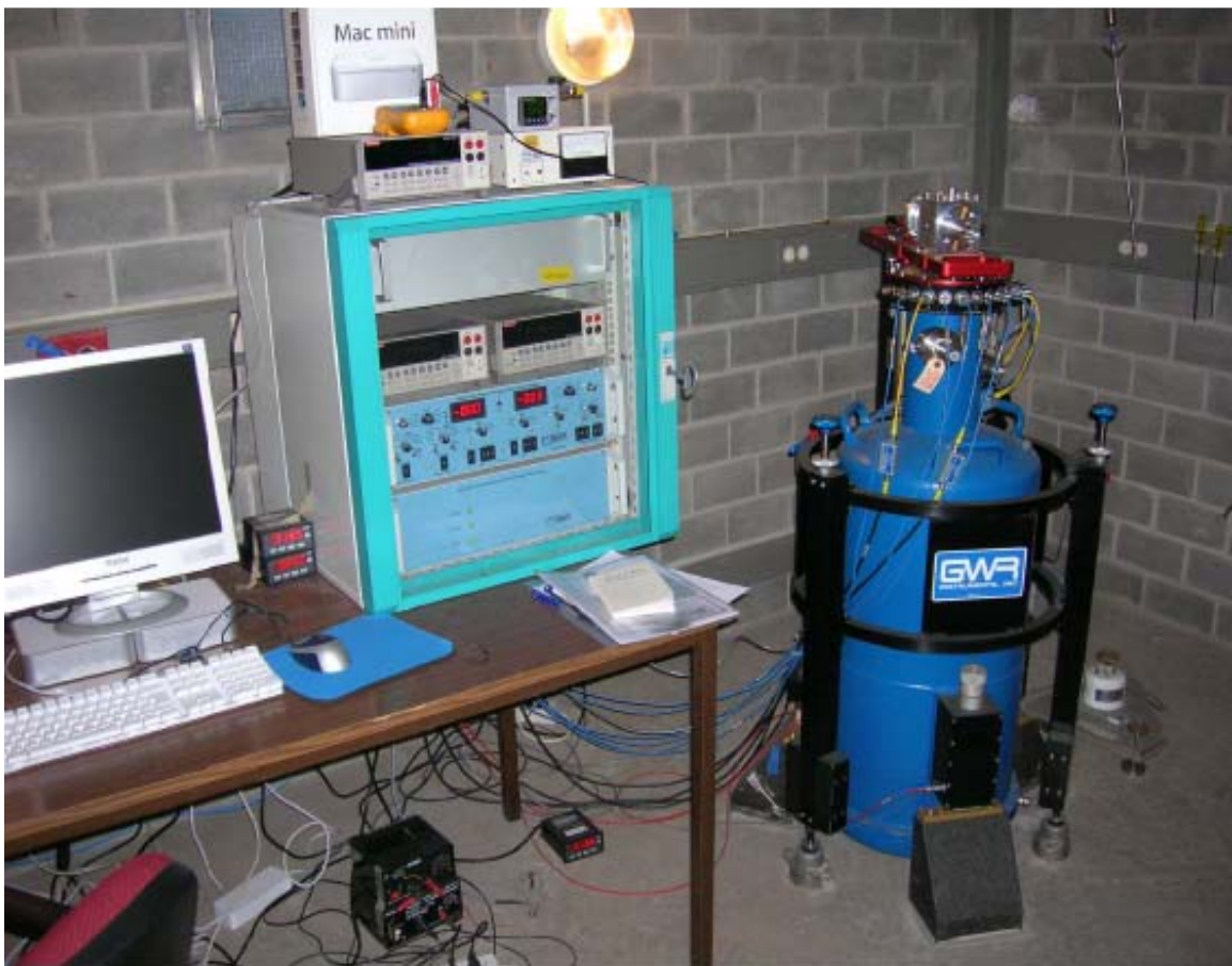
Fig. 3.10: The superconducting gravimeter OSGCT040 located in the Walferdange underground Laboratory for Geodynamics. The instrument provides high-resolution relative gravity measurements from the 19-12-2003.
