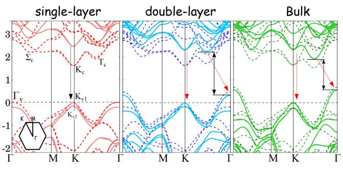
Conduction band is very sensitive to the crystal structure and to the GW "flavour"
