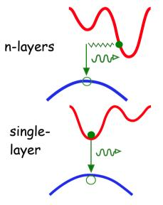
Direct/indirect bandgap depending on <u>number of layers</u> and <u>strain</u>
