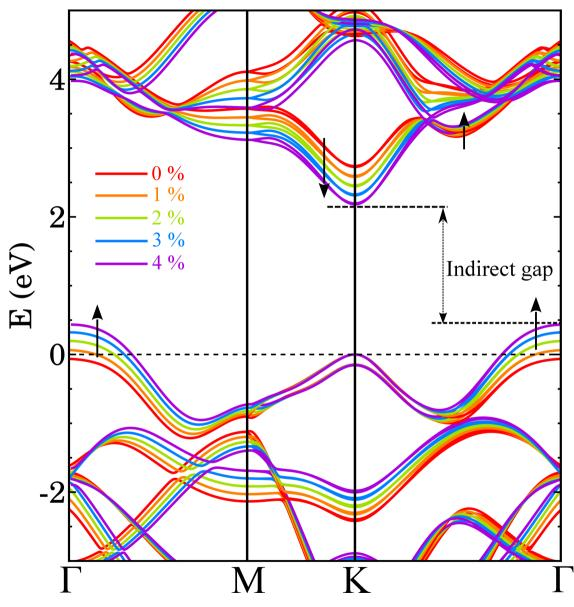
Strain changes the bandgap from direct to indirect
