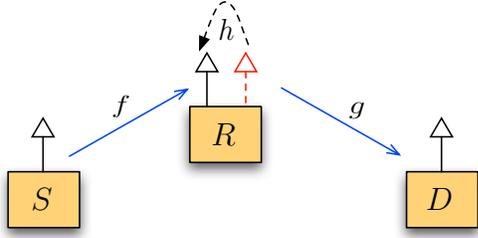
Fig. 1. The system model  $S \rightarrow R \rightarrow D$ ; the relay node employs a HU architecture (the second antenna at the relay node is used for the FD case).
