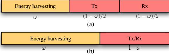
Fig. 2. Frame structure for HU-based AF: (a) HD relaying, (b) FD relaying.
