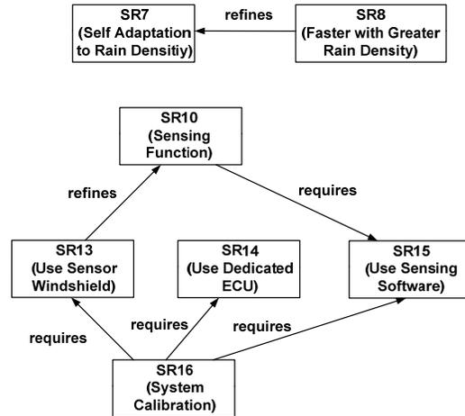
Figure 12 Changed Relations in the SysML Requirements Model
