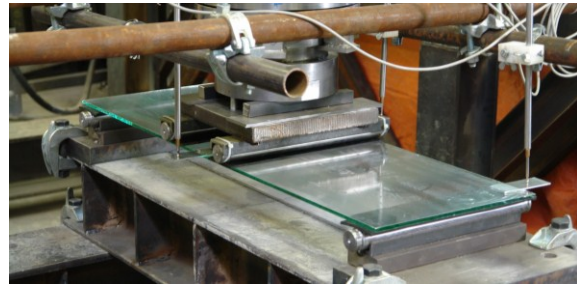
Figure 2.2- Four point bending test - EN 1288-3
