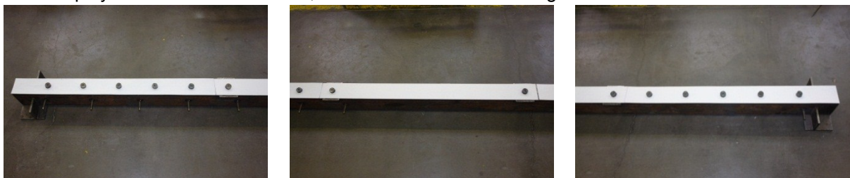
Figure 8.27- Repartition of the three Teflon plates fitting the welded steel studs of the mechanical adhesive connection
