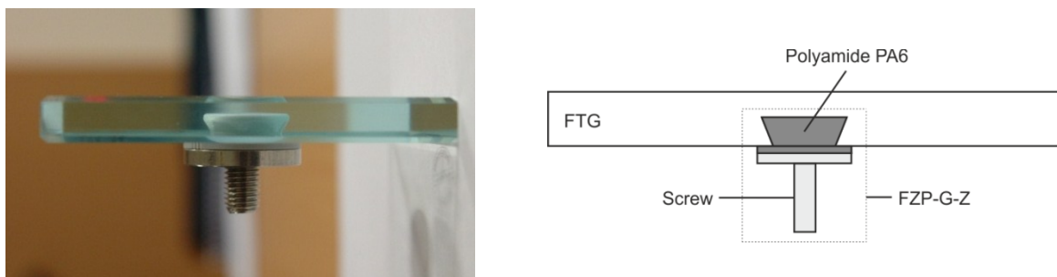
Figure 2.10- Undercut point fitting (Fisher FZP-G-Z) – General and detailed view
