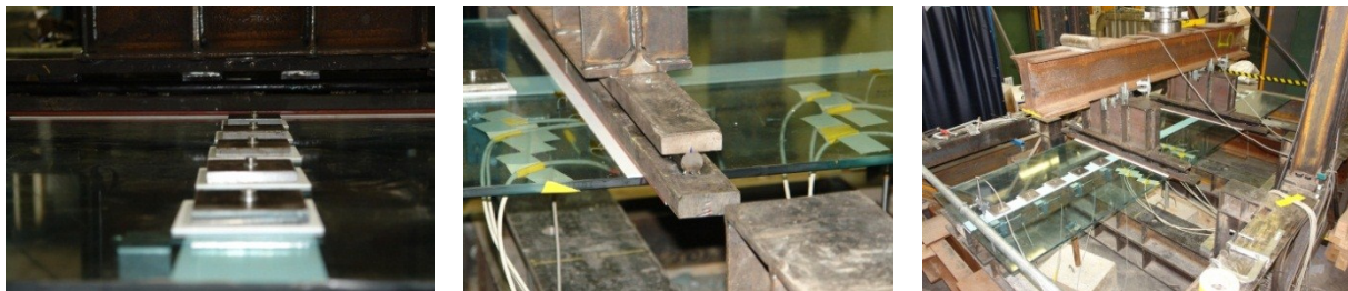
Figure 8.29- Test set-up for the large-scale mechanical adhesive beam tests and details of the system under the load
