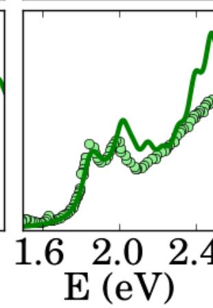
The exciton binding energy decreases with the number of layers. Consequence of larger dielectric screening. This compensates partially the GW correction.
