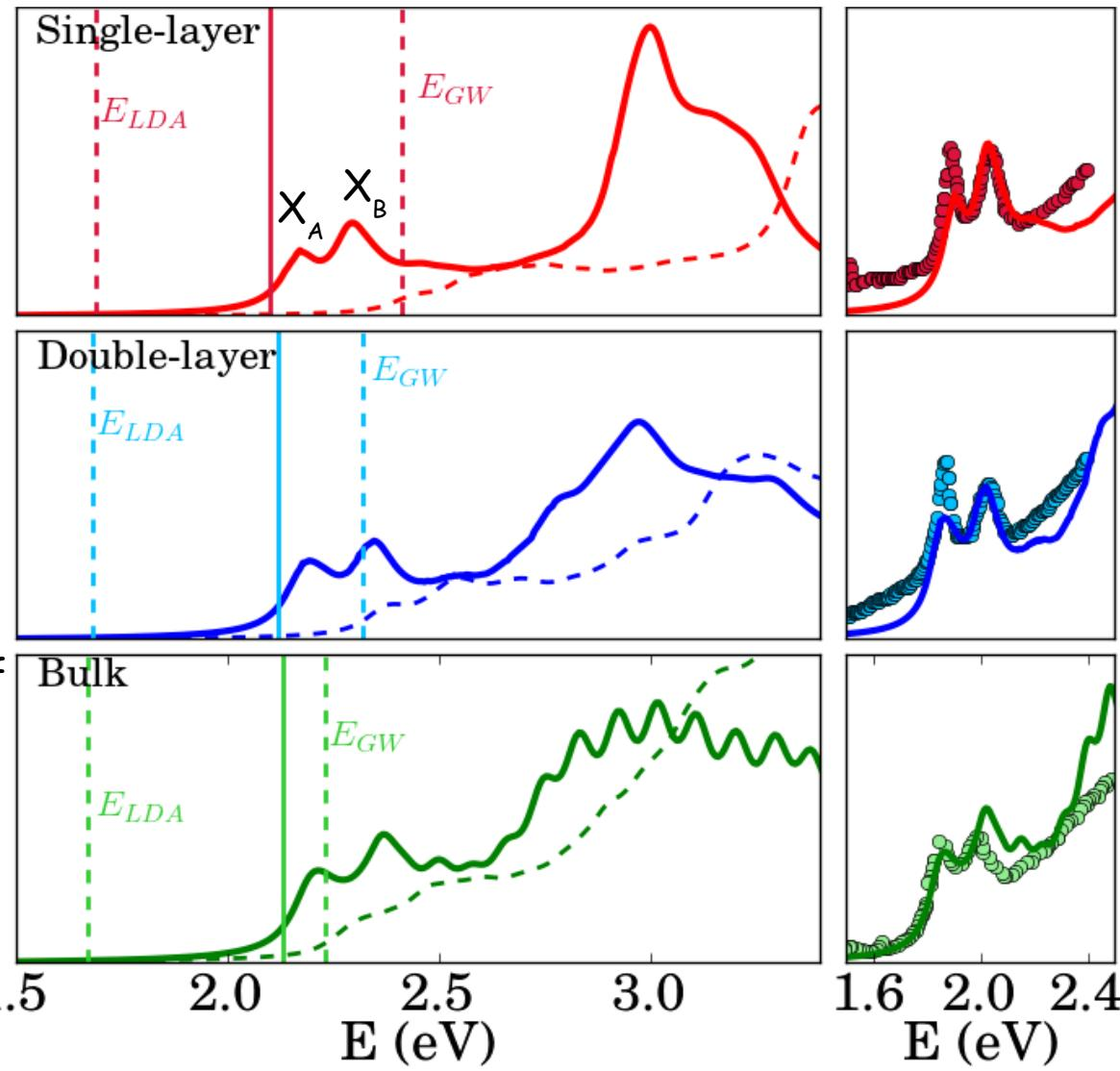
The exciton binding energy decreases with the number of layers. Consequence of larger dielectric screening. This compensates partially the GW correction.
