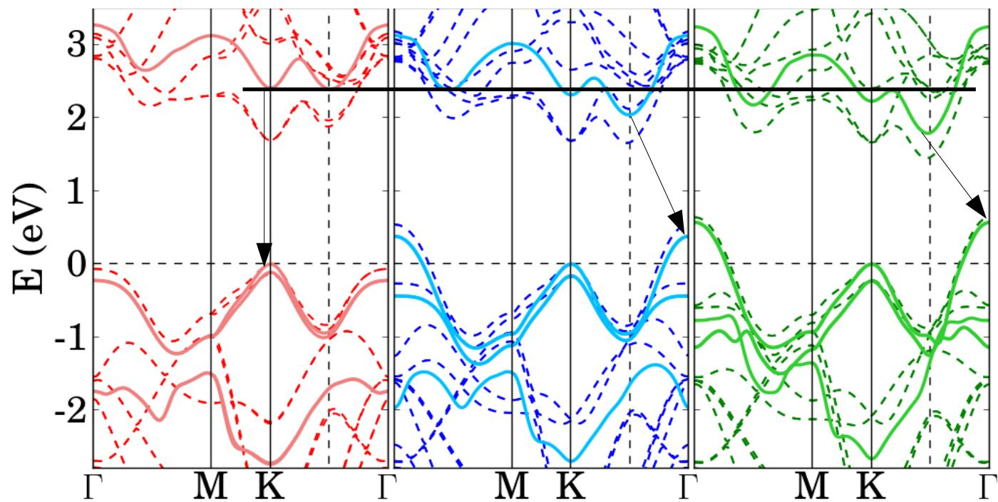
The addition of more layers changes the dielectric screening, the symmetry and the interlayer interaction.
