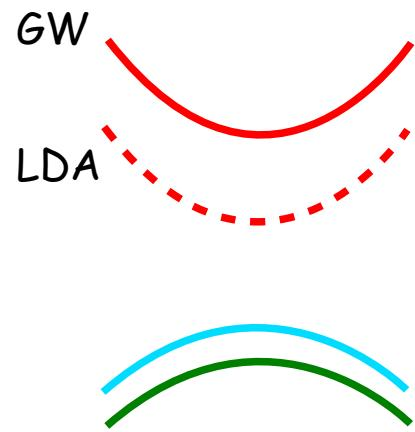
Correction of LDA bandgap underestimation by means of the GW method (spin-orbit interaction is included).
