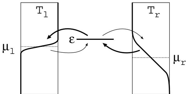
Fig. 1: Sketch of the nanothermoelectric engine consisting of a single quantum level embedded between two leads at different temperatures and chemical potentials. We choose by convention  $T_l < T_r$ . Maximum power is observed in the regime  $\varepsilon > \mu_l > \mu_r$ .
