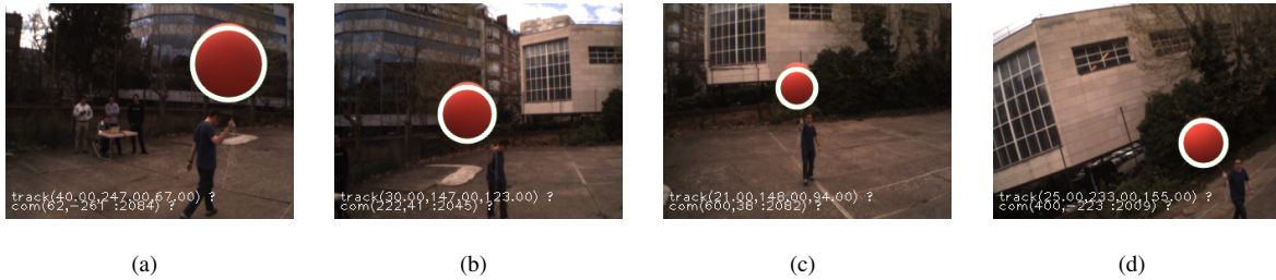
Figure 2: Camshift tracking of a colored red target on a image sequence. The white circle corresponds to the boundaries of the tracked colored area
