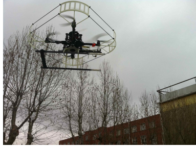
Figure 5: CVG-UPM [22] Pelican QuadCopter testbed used for sense and avoid experiments
