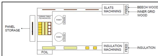
Figure 5 - Two Industrial robots and turning table solution
