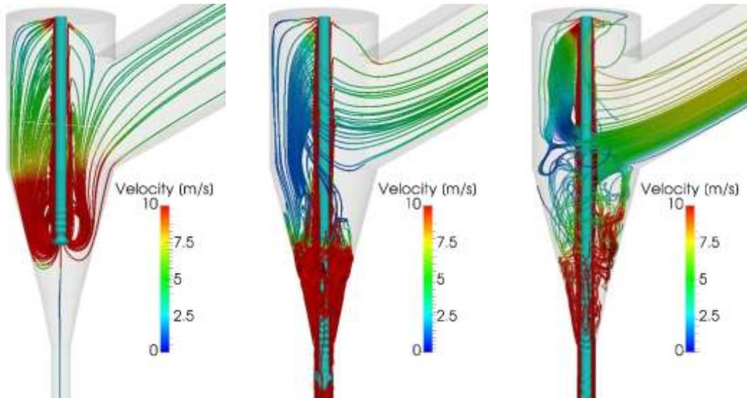
**Figure 2** Characteristic moment on the jet formation. Jet forming in the mixing chamber (left), Jet entering the tubular part (center), and fully developed jet (Right). The jet is colored in blue, streamlines of the velocity field are present
