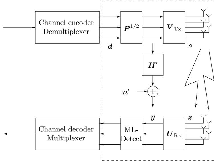
**Figure 13.1:** The components of a spatial multiplexing and loading MIMO system. In this chapter mainly the part within the dashed rectangle is considered.
