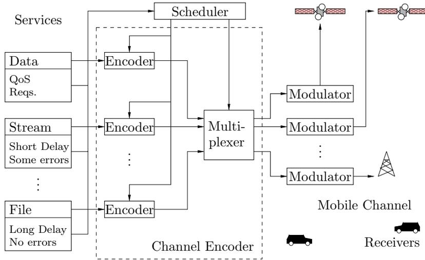
**Figure 2.1:** An end-to-end mobile satellite broadcast system with transmit diversity.
