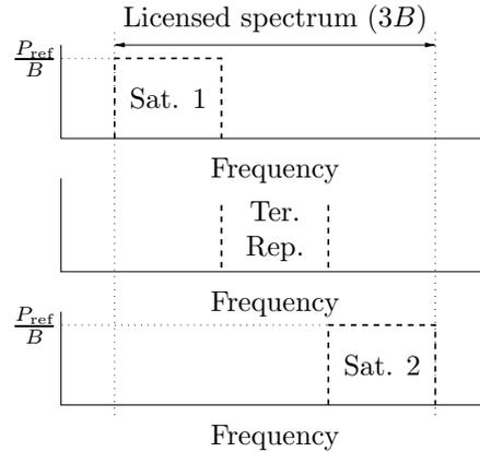
**Figure 3.3:** Reference single antenna, multiple frequency mobile satellite broadcast network. All transmitters transmit the same information (albeit possibly using different coding and modulation) for diversity. The y-axis illustrates the received signal power spectral density.
