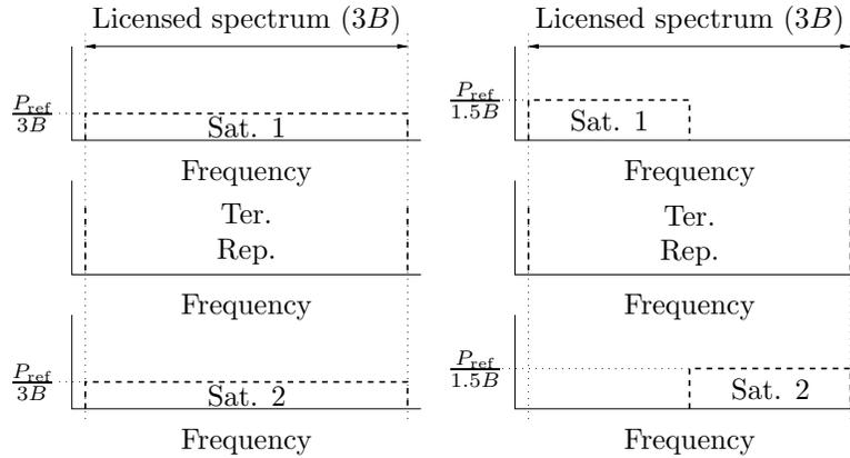
**Figure 3.4:** Bandwidth configuration in the two single frequency network configurations. The y-axis illustrates the received signal power spectral density.
