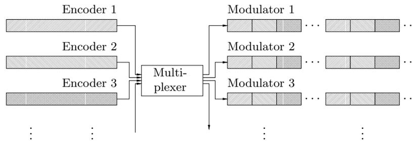
**Figure 2.2:** Principle operation of the multiplexer.
