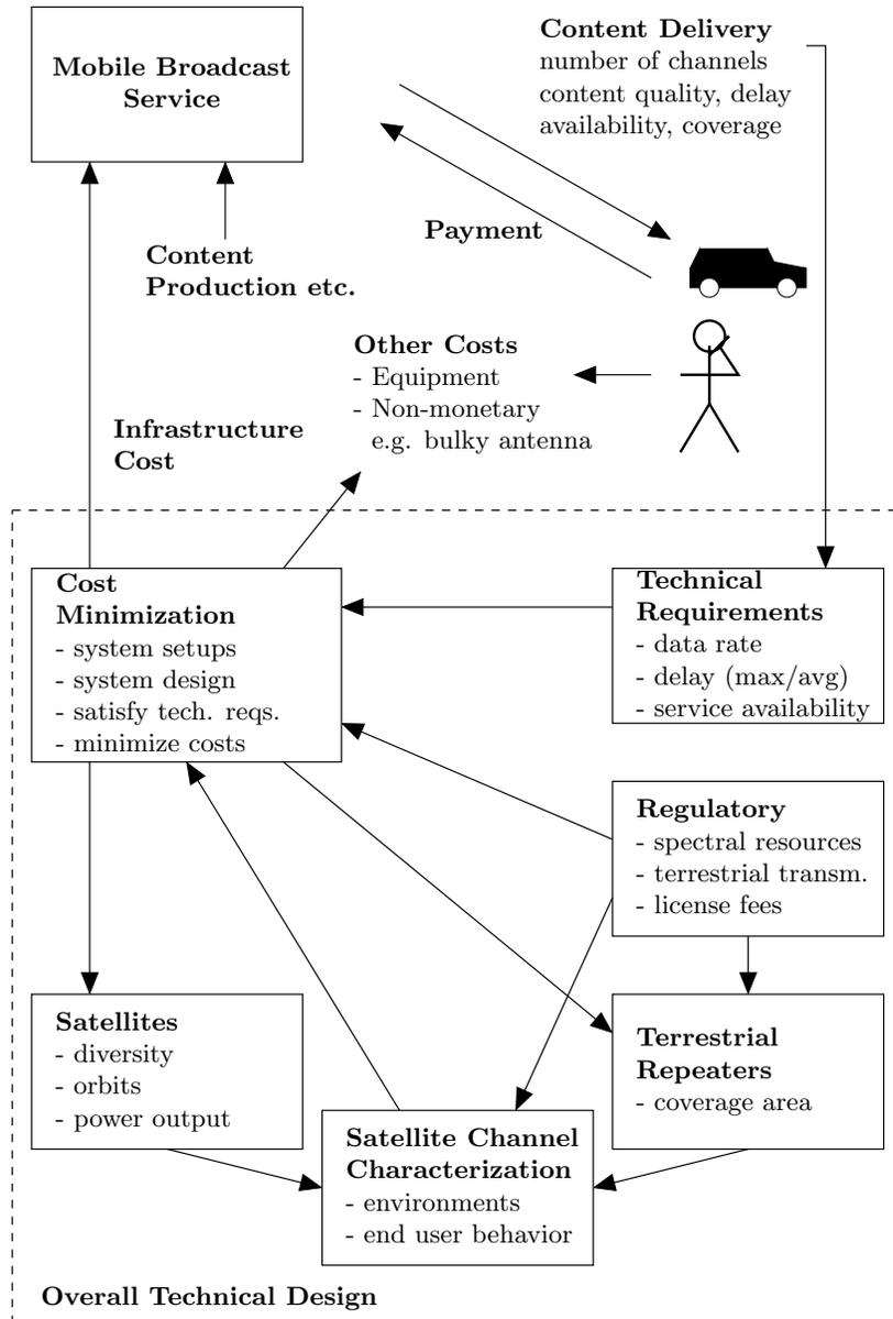
Figure 1.2: Design of a commercial mobile satellite broadcast system.
