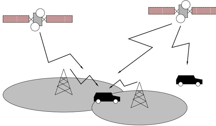
**Figure 3.2:** Example system setup consisting of  $s = 2$  simultaneously transmitting satellites and a network of terrestrial repeaters in a single frequency network configuration. The system is designed so that the transmitted data can be recovered even if only a single satellite signal is received.
