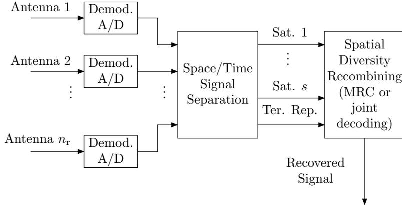
**Figure 3.6:** Principle functionality of an adaptive antenna single frequency satellite/terrestrial receiver.
