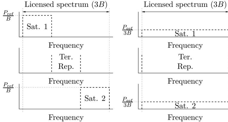
**Figure 3.5:** The example system in the two configurations considered for use with an adaptive antenna receiver. The y-axis illustrates the received signal power spectral density per receive antenna.
