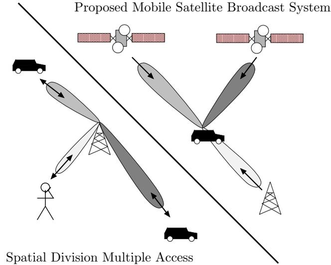
**Figure 3.7:** Comparison of spatial division multiple access and the adaptive antenna, single frequency broadcast network proposed in this chapter. Note that the broadcast network only requires directive reception and since the different signals contain identical information they can be recombined to improve performance.
