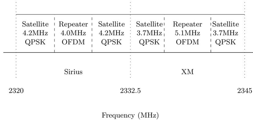
**Figure 3.1:** Frequency band allocation and use for the US mobile satellite broadcast systems [FJK<sup>+</sup>02].
